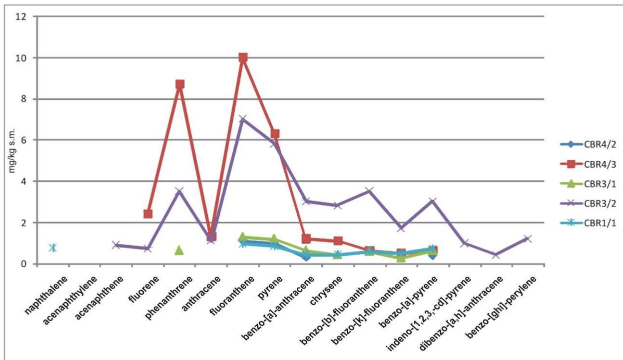
Fig. 8. The results comparison of PAHs analysis in soil samples
