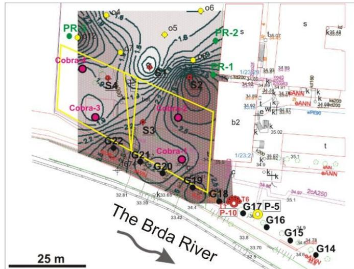
**Fig. 2. Research area embankment - isopachous line map**
