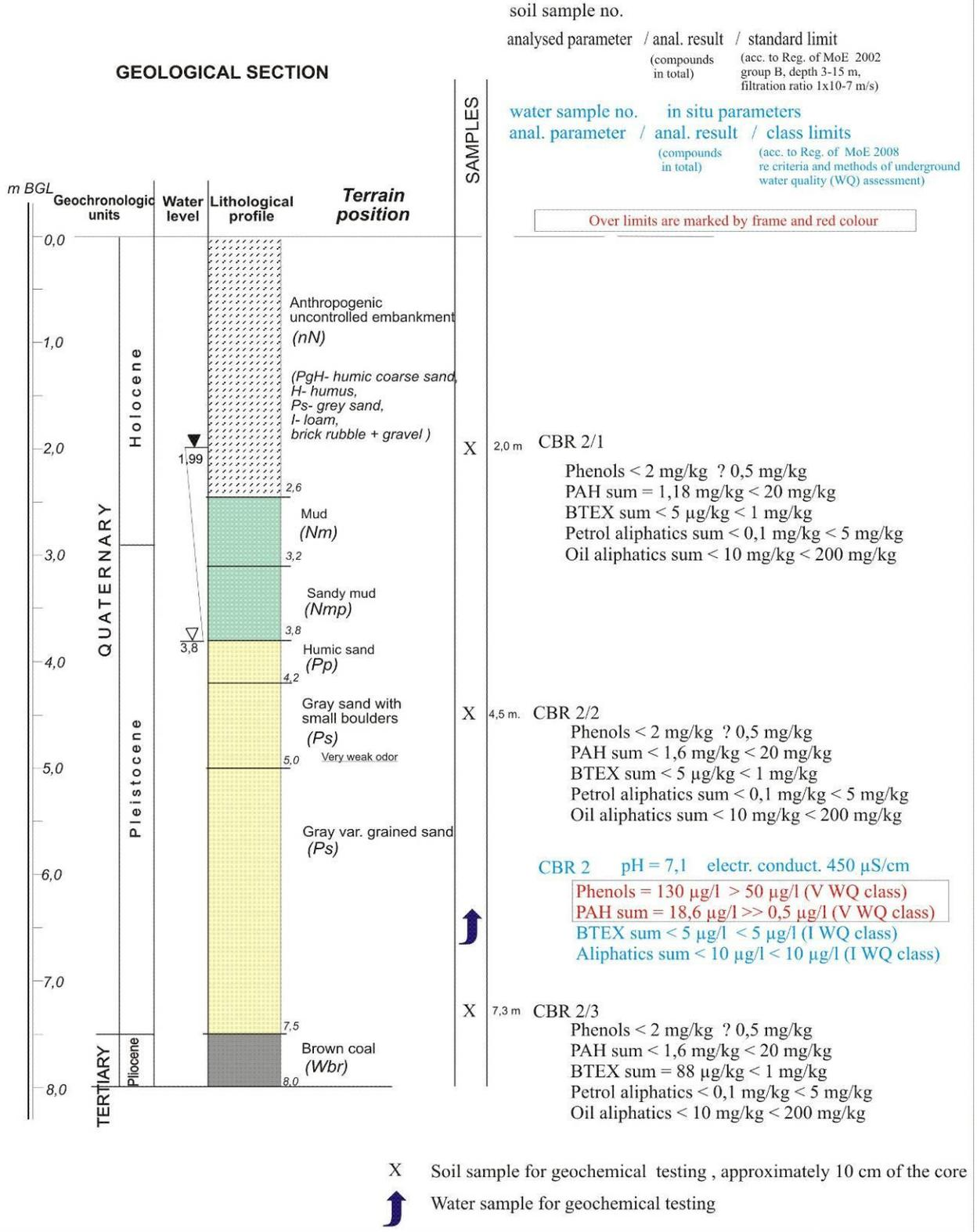
Fig. 5. Geological and chemical profile of Cobra-2 borehole
