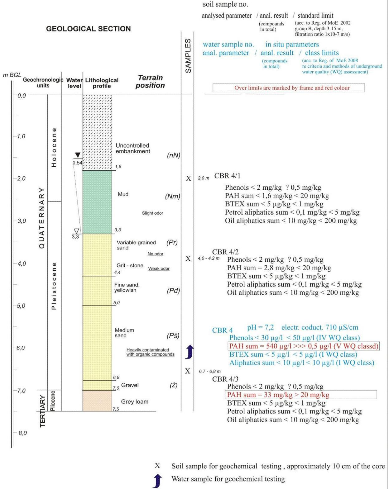
Fig. 7. Geological and chemical profile of Cobra-4 borehole
