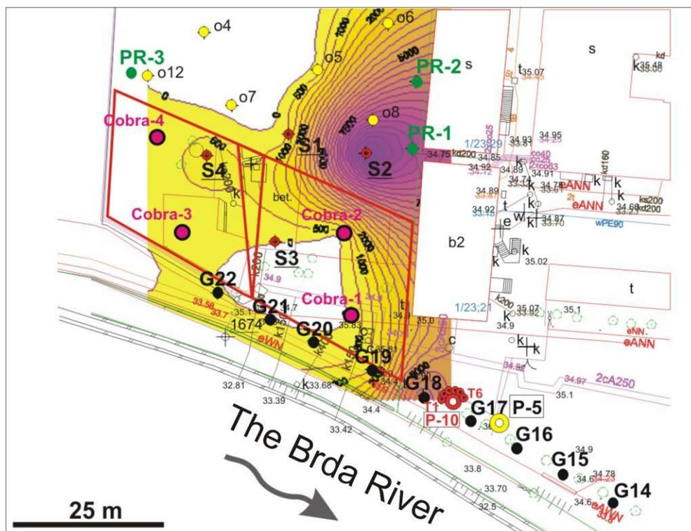
Fig. 13. Contents of total PAHs (in  $\mu\text{g}/\text{l}$ ) in groundwater, sampling on depth of 6,5 m
