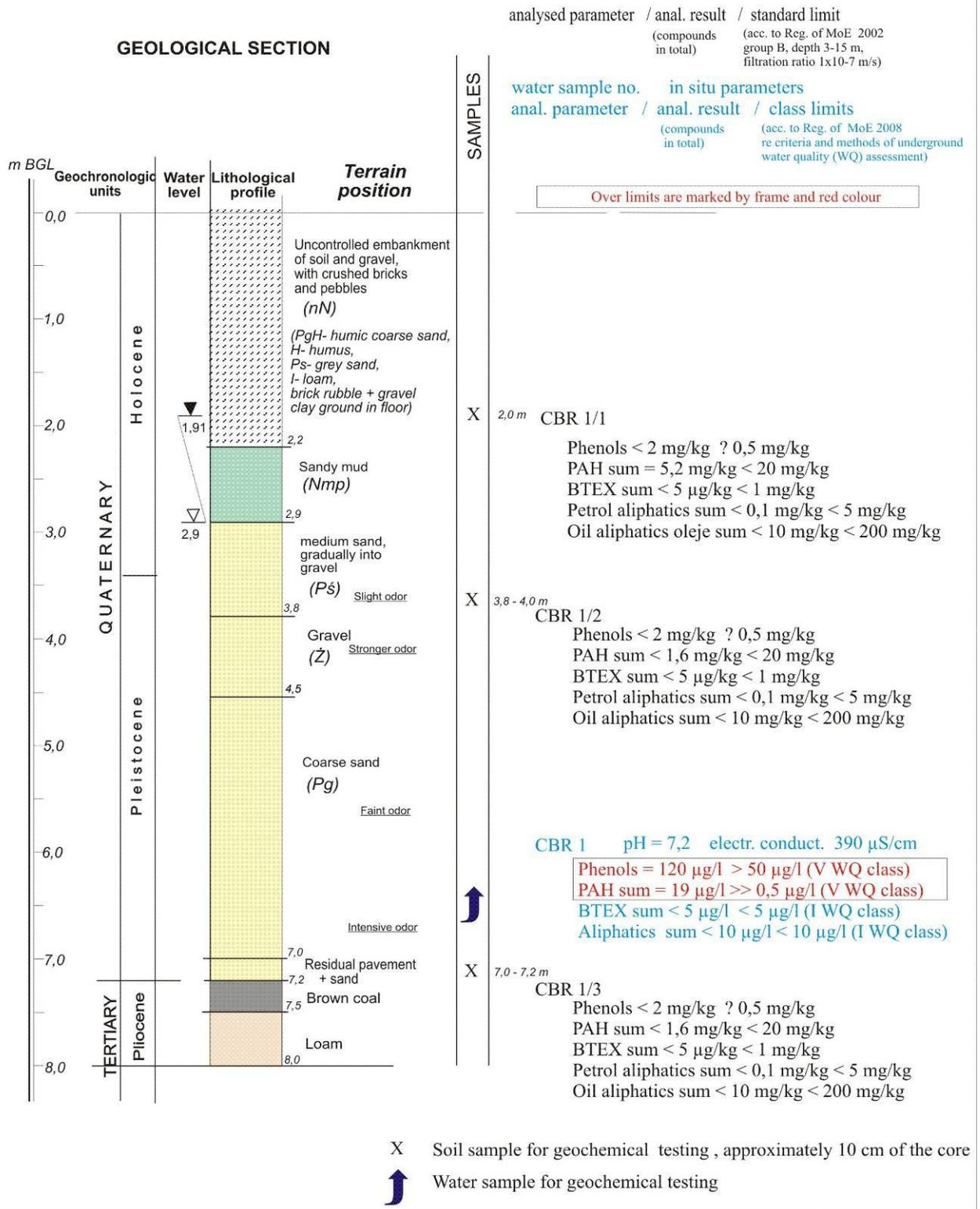
Fig. 4. Geological and chemical profile of Cobra-1 borehole
