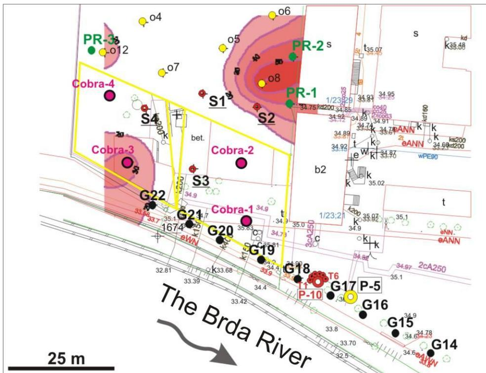
Fig. 11. The contents of total PAHs (mg / kg dm) at a depth of c.a. 4 m.. The first contour line - 20 - is the limit allowable concentration value for the grounds of group B.
