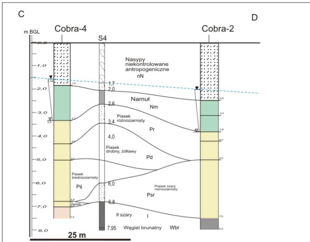
nN– uncontrolled anthropogenic embankment, Nm– mud, Pr - variable grained sand, Pd-fine sand, Pś- medium sand, Pśr – grey variable grained sand, Żwerek – Grit stone, I – grey loam, Wbr – brown coal;
