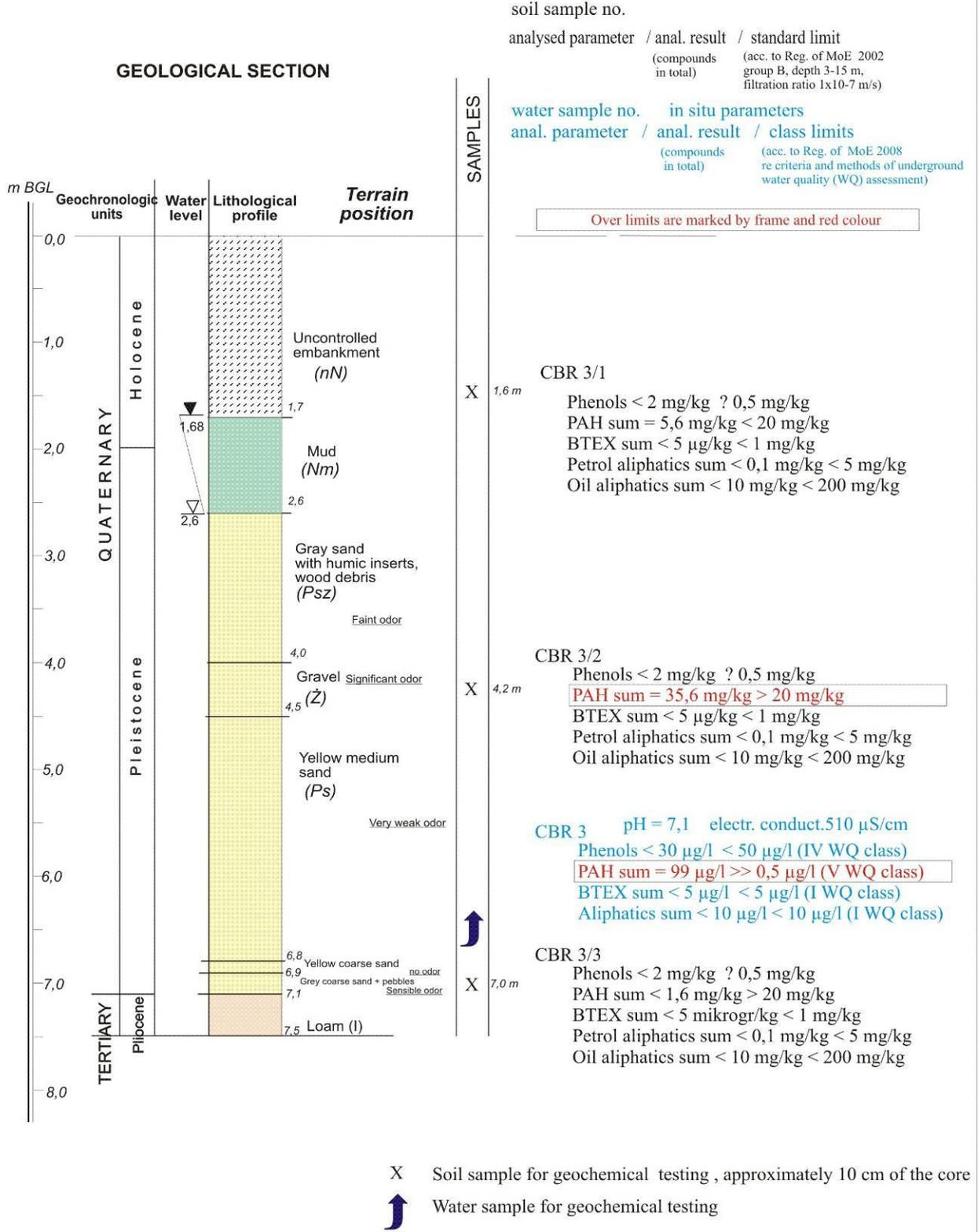
Fig. 6. Geological and chemical profile of Cobra-3 borehole
