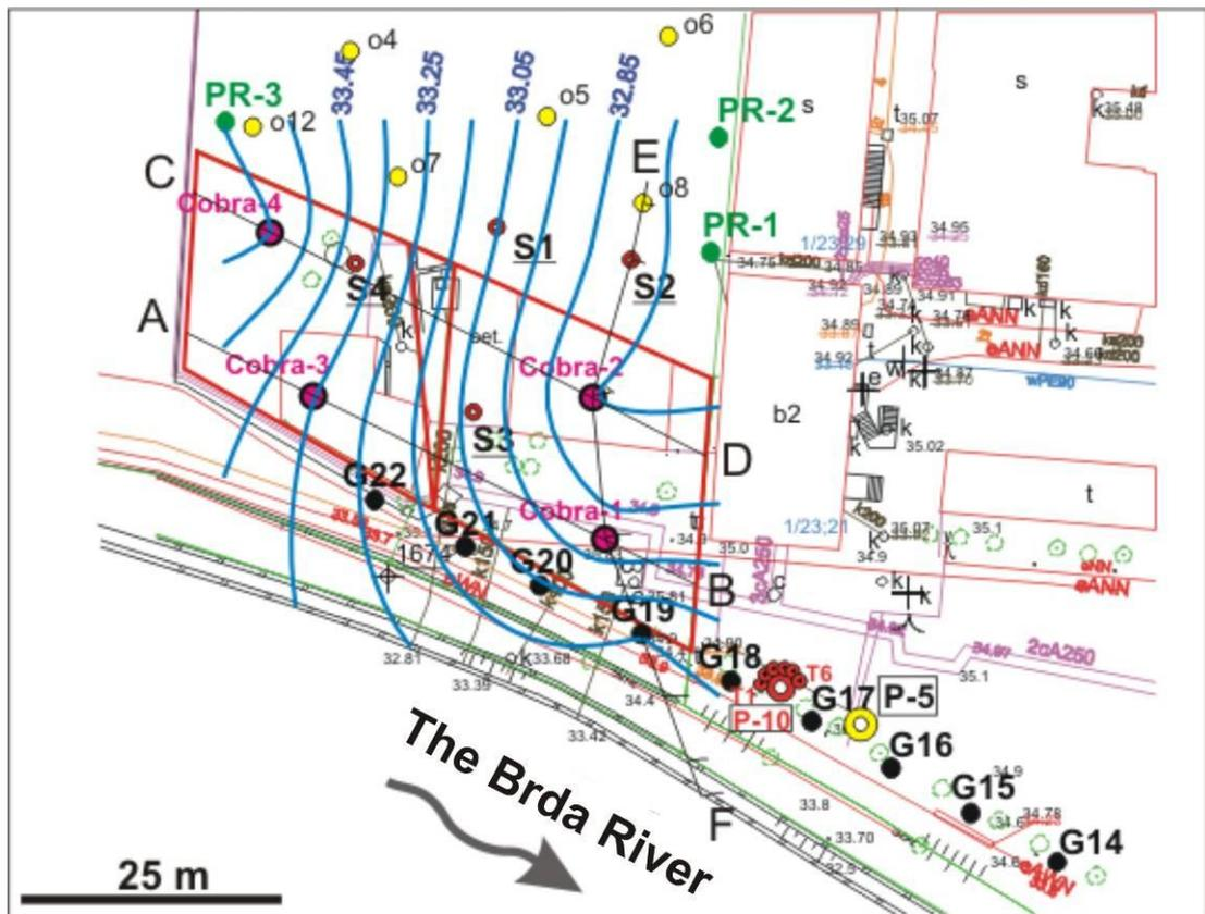
Hydro-isohypses of the underground water level from the first aquifer, remaining in the clear hydraulic communication with the Brda River. Situation from 9<sup>th</sup> of June 2010. Lines of sections are marked: AB, CD and EF.
