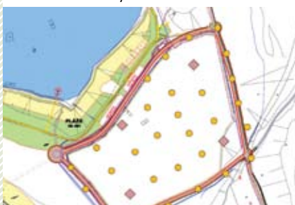
Area of the geotechnical survey with the locations of probes
