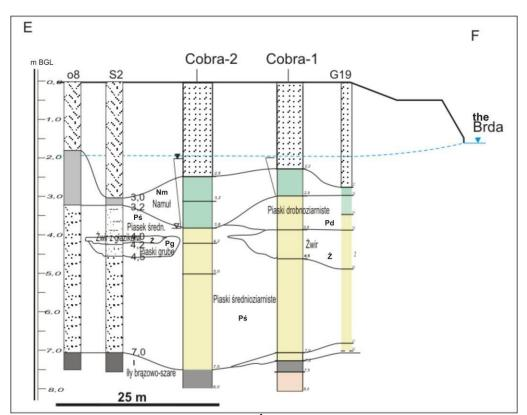
Nm- mud, Pd-fine sand, Pś- medium sand, Ż- gravel, Pg- coarse sand, I- brown-grey loam;
