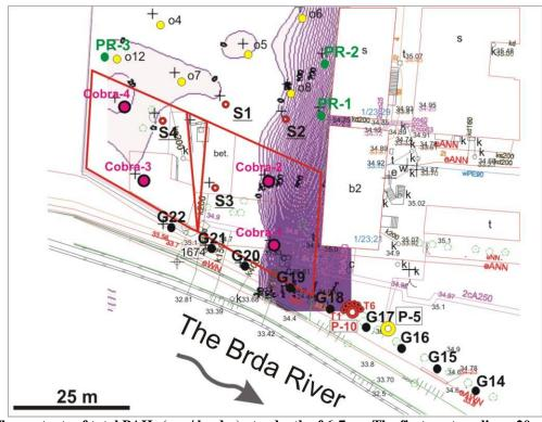
Fig. 12. The contents of total PAHs (mg / kg dm) at a depth of 6-7 m.. The first contour line - 20 - is the limit allowable concentration value for the grounds of group B.
