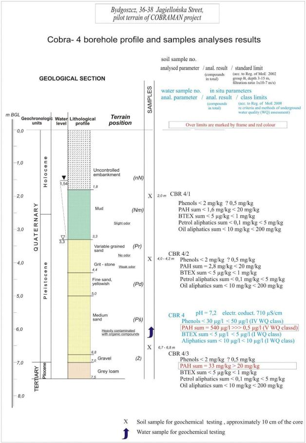
Fig. 7. Geological and chemical profile of Cobra-4 borehole
