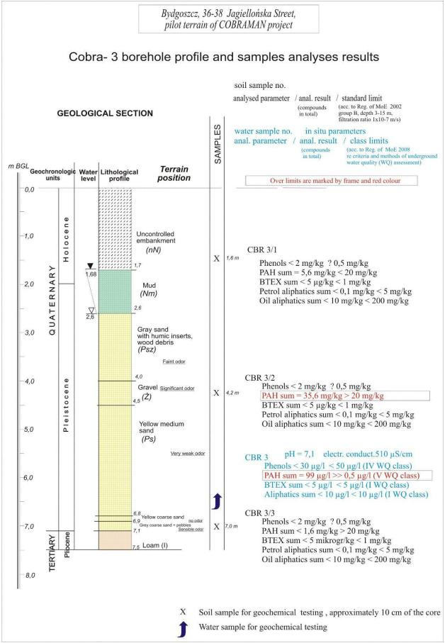
Fig. 6. Geological and chemical profile of Cobra-3 borehole
