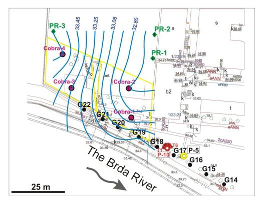
Fig. 1. Hydro-isohypses on research area on 9th of June 2010
