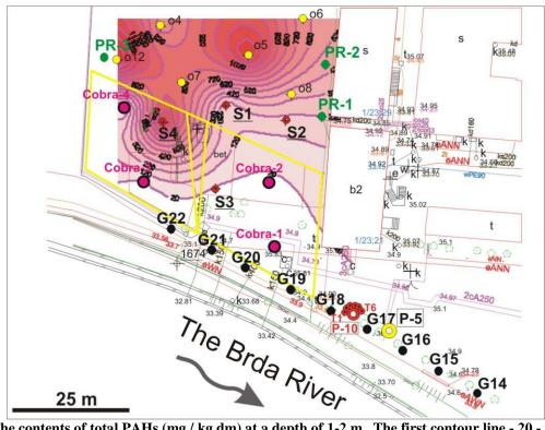
Fig. 10. The contents of total PAHs (mg / kg dm) at a depth of 1-2 m.. The first contour line - 20 - is the limit allowable concentration value for the grounds of group B.
