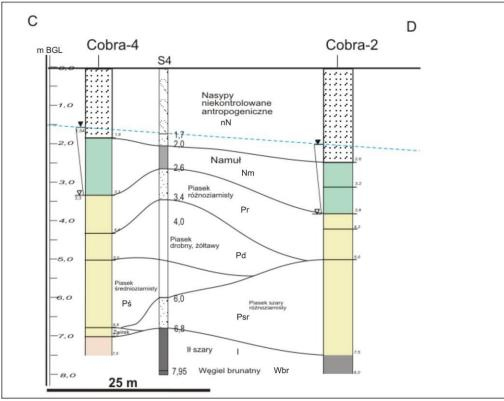
nN– uncontrolled anthropogenic embankment, Nm– mud, Pr - variable grained sand, Pd-fine sand, Pś- medium sand, Psr – grey variable grained sand, Żwirek – Grit stone, I – grey loam, Wbr – brown coal;
