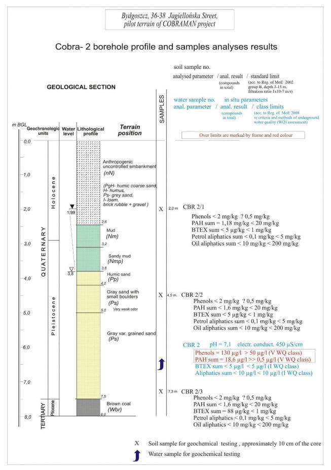
Fig. 5. Geological and chemical profile of Cobra-2 borehole
