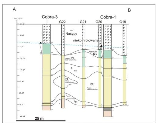
nN- uncontrolled embankment, Nm- mud, Pd-fine sand, Ż-gravel, Pś- medium sand, Pg- coarse sand;
