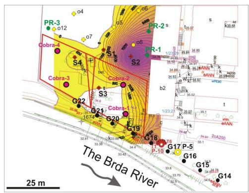
Fig. 13. Contents of total PAHs (in µg/l) in groundwater, sampling on depth of 6,5 m
