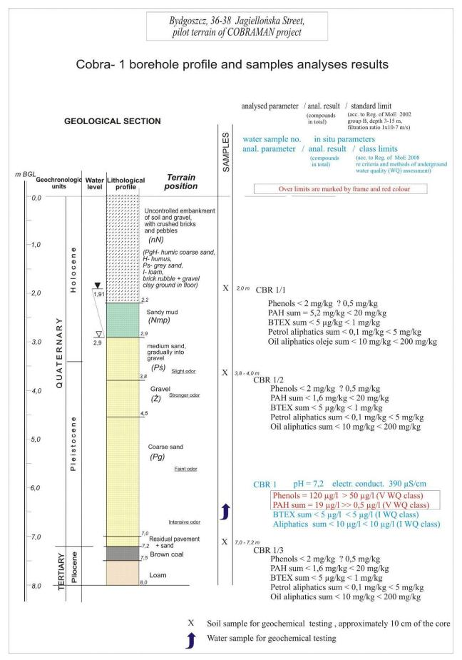
Fig. 4. Geological and chemical profile of Cobra-1 borehole
