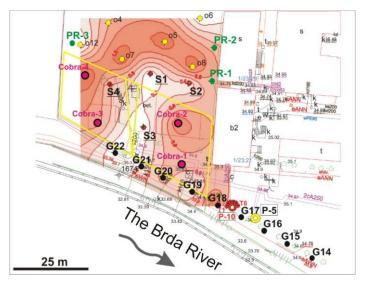
Fig. 3. Research area alluvium - isopachous line map
